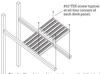
**Step 1-** Place 1st panel into step beams at far left side of shelf. Position panel so required transverse flue space is maintained between left edge of panel and shelf in adjacent rack bay.
